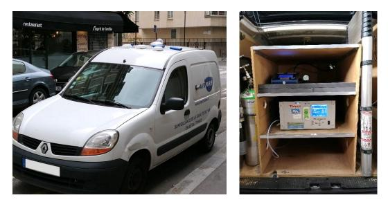
Figure 4: Airparif vehicle equipped for mobile evaluation. External view of vehicle setup (left) and detail of internal setup (right).
