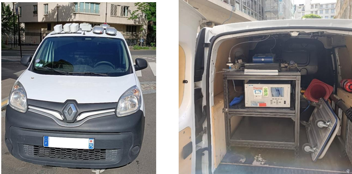
Figure 4: Airparif vehicle equipped for mobile evaluation. External view of vehicle setup (left) and detail of internal setup (right).
